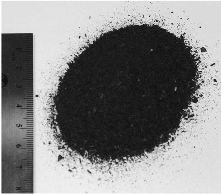
Figure 1. Photograph showing the texture and size of the dried pavement sealant flakes as prepared and used in this study.
